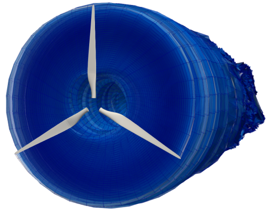
Figure 2. Panel method simulation results of the UNAFLOW rotor and its wake.
