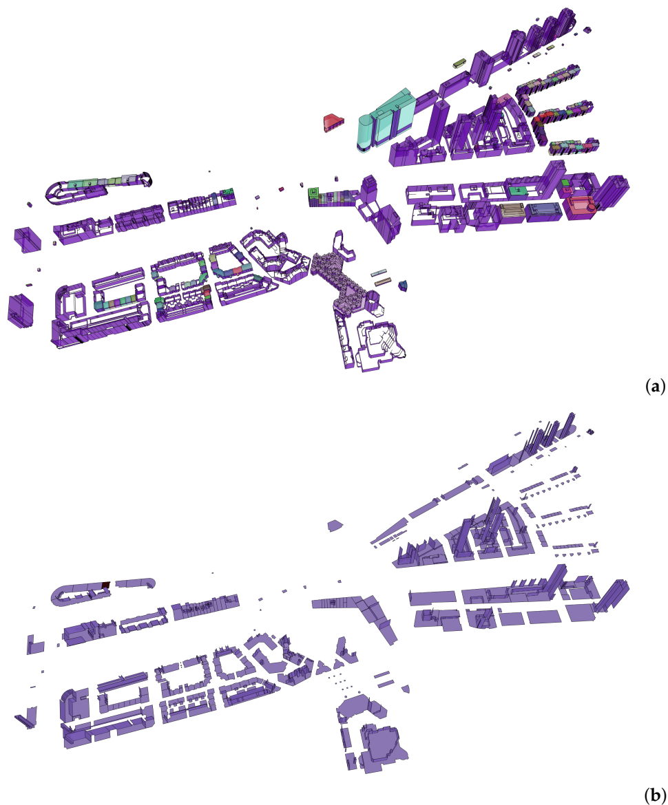
Figure 11. Result of FME conversion visualized in RDF IfcViewer. (a) IfcWalls in purple and IfcSpaces with various colours; (b) IfcSlabs.
