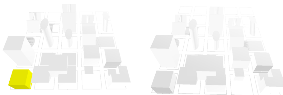
Figure 3. Case B: IFC geometries, both in IFC v.2x3 and v.4, converted to bldg:buildings , visualized in azul. It is possible to notice that, for some reason, these are inverted with respect to their original distribution.
