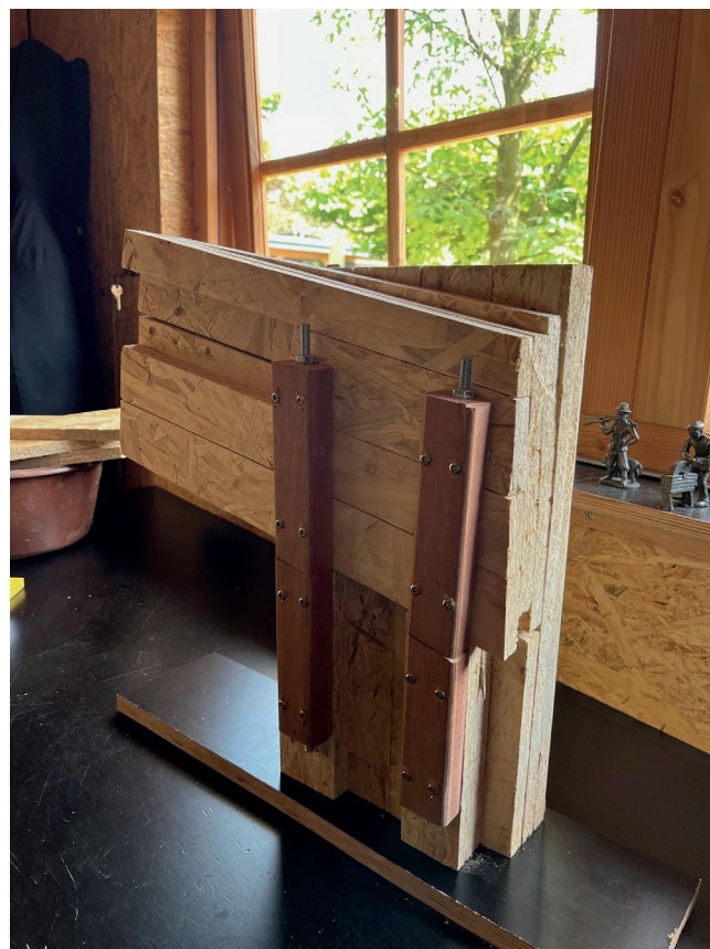
Figure 6.25: mock-up of moment connection
