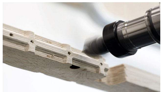
Figure 2.15: three dimensional male-female shear connection Kunic, A., & Naboni, R. (2023b)
