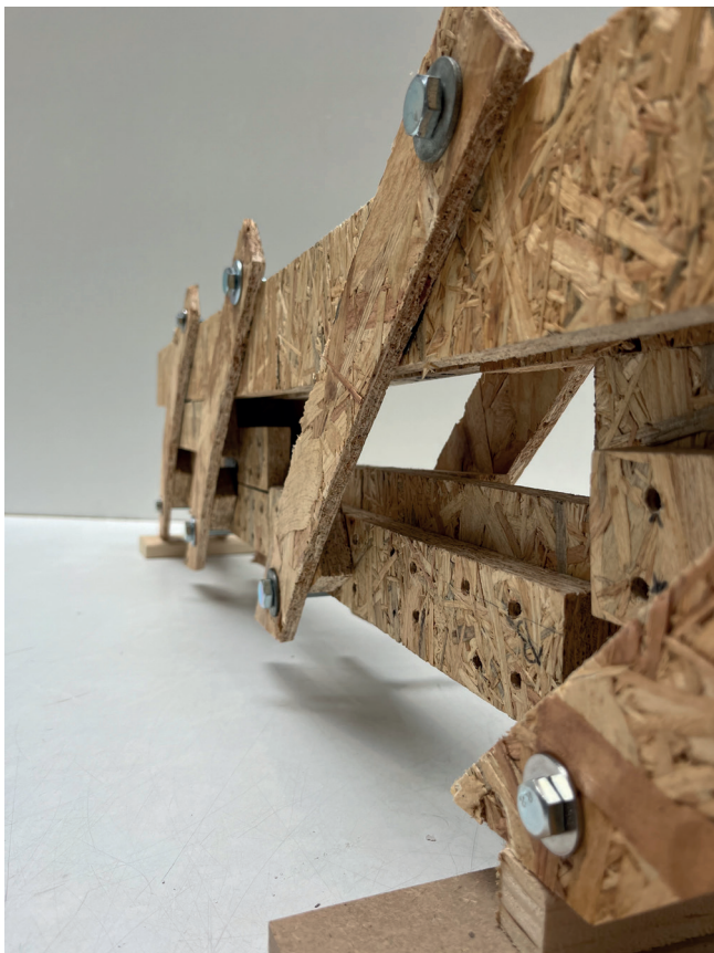
Figure 8.34: close up on optimised parts showcasing the link and spacing block
