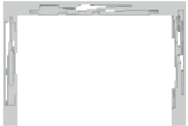
Figure 8.37: Optimised geometry with exaggerated large cross-section using varying strength grades C14 - C30.
