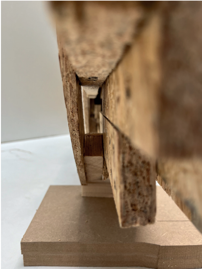
Figure 8.32: Close up of build section highlighting deformed clamp and the spacing block
