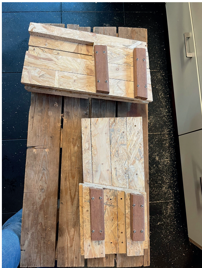
Figure 6.23: mock-up of moment connection
