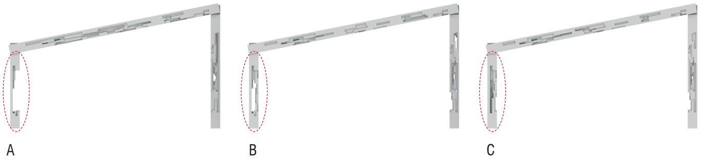
Figure 8.36: Buckling behaviour found in the algorithm, A). Optimised structure without accounting for buckling. B). Buckling factor of 1.1. C). Buckling factor of 1.28.
