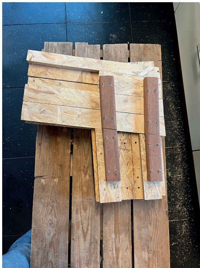
Figure 6.24: mock-up of moment connection
