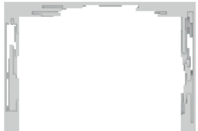
Figure 8.38: Optimised geometry with exaggerated large cross-section using varying strength grades C24.
