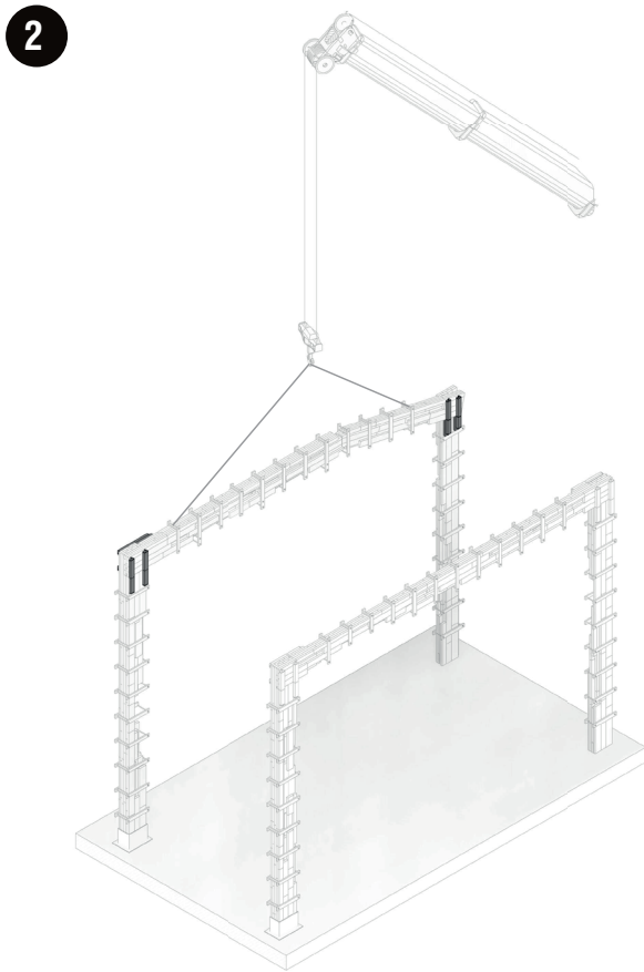
Figure 9.23: Construction phase 2: Fastening the elements in place
