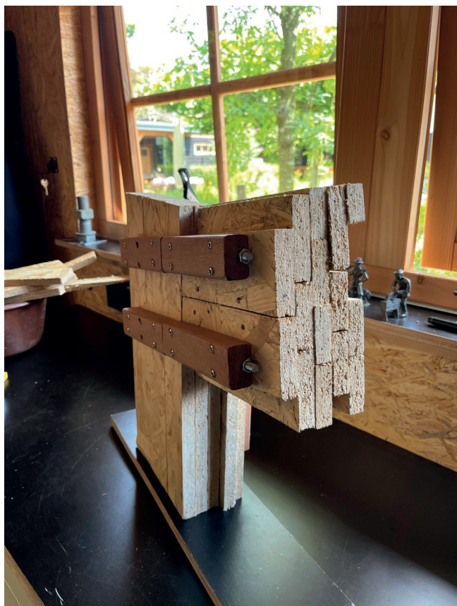
Figure 6.24: mock-up of moment connection
