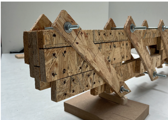
Figure 8.28: Mock-up highlighting clamping system
