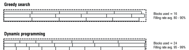
Figure 7.2: Result of piece placement only considering the X-direction without any constraints, Greedy search method compared with a Dynamic programming method.
