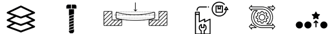
Figure 6.2: design criteria, from left to right: Massive layering, reversible joints, ductile system, minimize re-fabrication, tectonic flexibility and use of unique parts.
