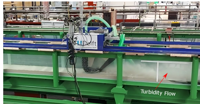
Figure 5. An experimental run in progress showing the turbidity flow generated behind the collector head.
