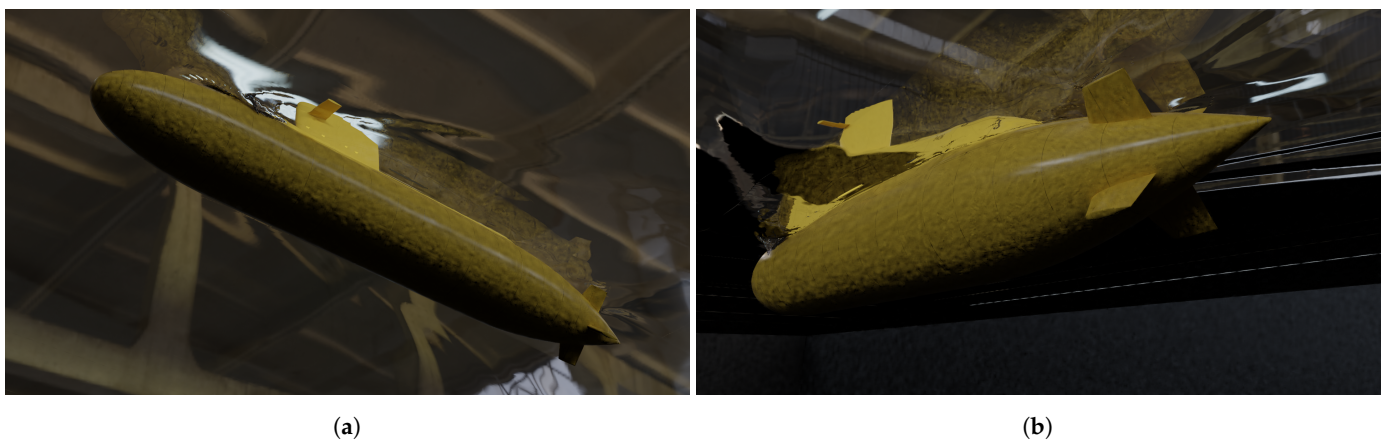
Figure 9. BB1 submarine Blender visualisation below the water surface, focused on (a) the bow and (b) the stern. Free-surface extracted using an air volume fraction iso-contour of 0.5.
