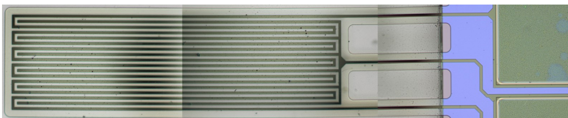
Figure 8.20: Device 2, group 3. No signs of delamination, void formation, corrosion, or mechanical damages.
