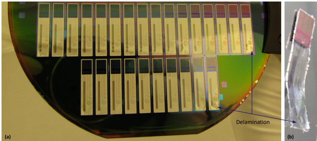
Figure 8.12: Parylene encapsulation delamination on the devices located at the edges of the wafer. (a) Affected devices in a wafer frame. (b) Released device with delaminating parylene layers.
