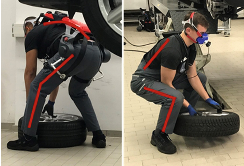
Fig. 1. Body postures while picking up a wheel with (left) and without active exoskeleton “Cray X” (right).
