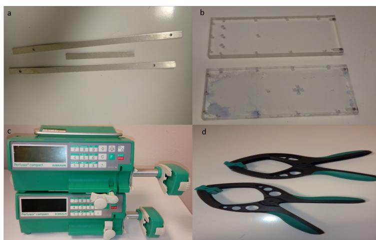
Figure 3.6: a)The Aluminium spacers used to separate the plates b)The plexi-glass plates c)Syringe pumps used to deliver fluid into the set-up d)The clips used to suppress the plates.
