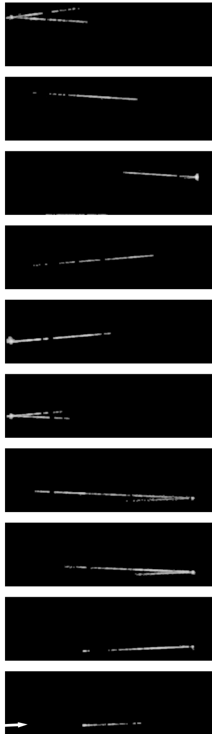
Figure 3. Images of the travelling laser pulse captured at the frame interval of 10 ns (from the bottom to the top). Much higher spatial resolution is achieved by the silicon image sensor than most of past light-in-flight imaging, except holographic images by Kubota and Awatsuji [2,3].
