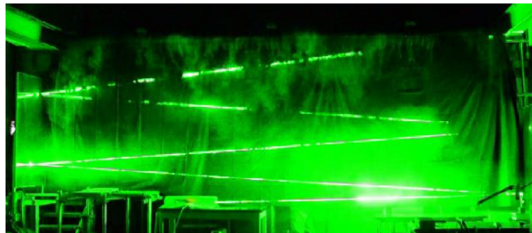
Figure 2. Front-side experimental set-up and a frame with a laser beam taken by a consumer video camera (a) The set-up includes three fog machines on the stage, a pair of mirrors, a small mirror for high-power laser beam reflection and adjustment of the direction of the laser beam, a laser and a backside curtain. The camera and timing controllers are placed on the other side. (b) The frame is extracted from images taken with a consumer video camera. Other frames are completely dark. Fog released at the second emission is falling over the stagnated fog generated after the first release.
