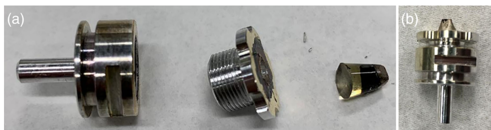
FIGURE 1 In-house made sample holder for serial slice and view (SSV) characterization of trimmed blocks contacting bone pieces
