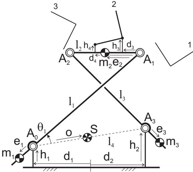
Fig. 2. Design parameters and link masses  $m_i$  for force balance with the common CoM in  $S$  for any motion of the mechanism.
