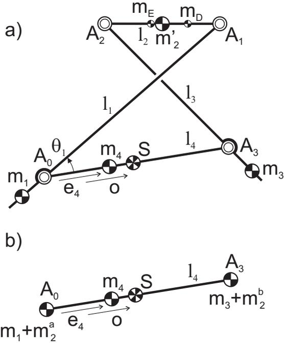
Fig. 8. Calculation of the common CoM in  $S$  with the mass  $m_4$  of the link  $A_0A_3$  included.
