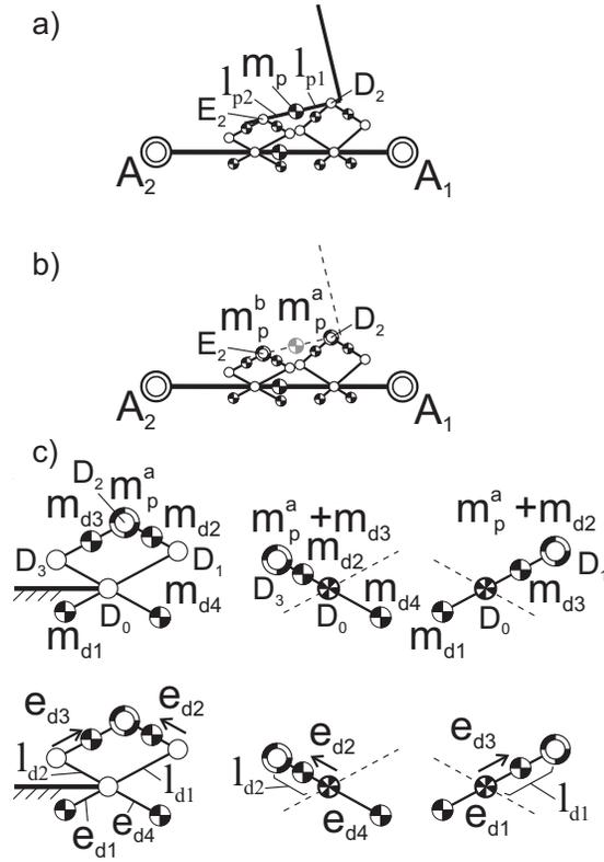
Fig. 6. Mass equivalent models of the coupler link design with its two reconfiguration mechanisms for deriving the force balance conditions.
