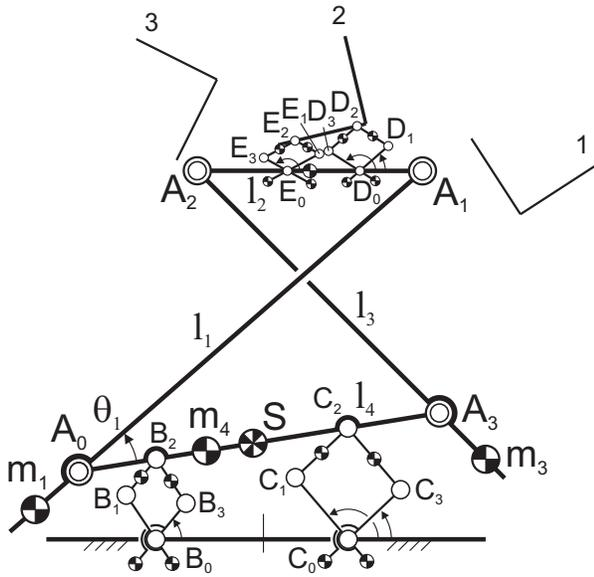
Fig. 4. Design of a force balanced reconfigurable four-bar linkage with four balanced 2-DoF parallel manipulators to relocate the base pivots and to relocate the coupler pivots for an end-effector motion through a different set of three desired poses.
