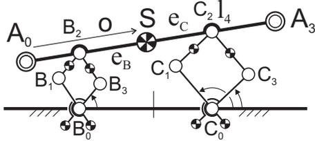
Fig. 9. Design of the base link with its two reconfiguration mechanisms of which the balance conditions can be derived in the same way as illustrated in Fig. 6.
