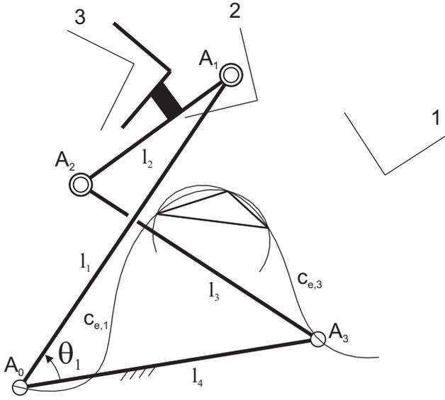
Fig. 1. 4R four-bar mechanism with base link  $A_0A_3$  obtained from three-position synthesis when the end-effector on coupler link  $A_1A_2$  passes through the three defined poses with the link lengths given [4].
