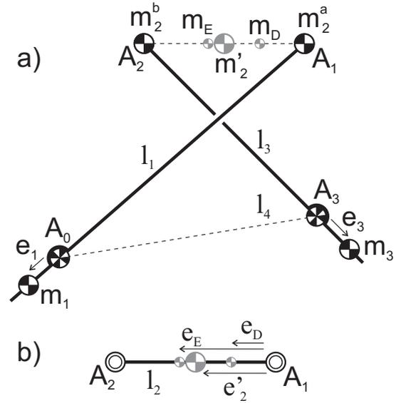
Fig. 7. Mass equivalent model of the four-bar linkage design for deriving the force balance conditions.
