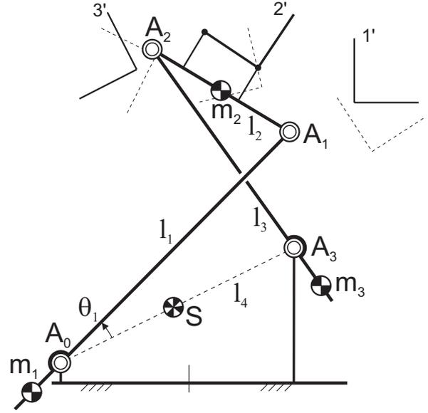
Fig. 3. Reconfigured force balanced four-bar linkage for a different set of three desired task poses with the same link lengths and mass distributions and with different locations of base pivots and of coupler pivots.
