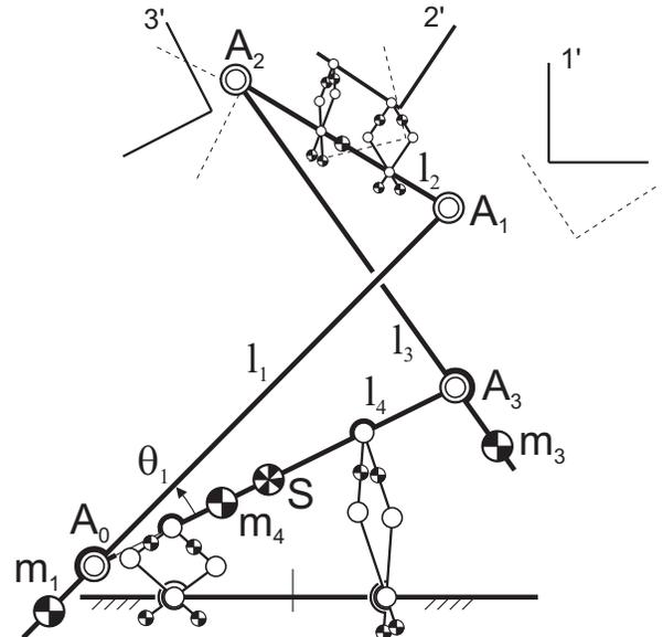
Fig. 5. Example of the relocation of the base pivots and the coupler pivots by the four reconfiguration mechanisms for the new set of three task poses.
