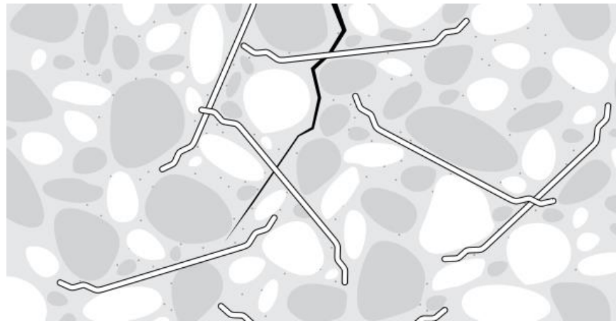
Figure 2.8 Steel fibres in a concrete mixture bridging a crack (Bekaert, 2013).
