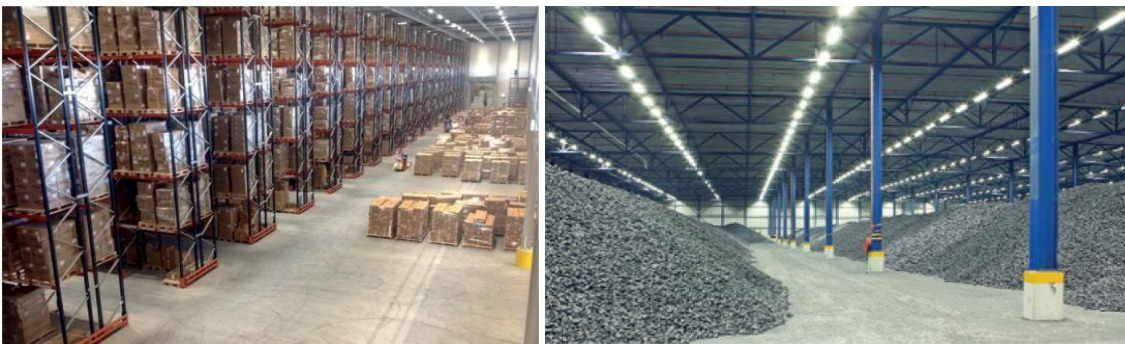
Figure 1.4 Typical floor loadings. Left: a racking warehouse. Right: bulk storage. Figures adapted from (Loonen N. , 2018).
