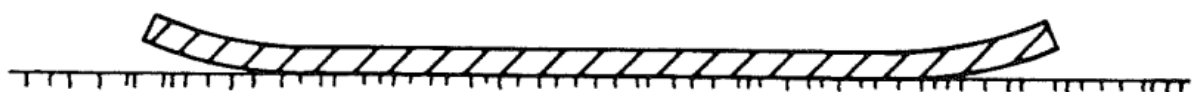
Figure 3.4 A shrinkage gradient in a jointless floor causing the free ends to curl upwards which will be restrained due to the self-weight.
