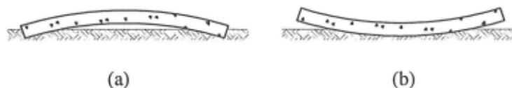
Figure 3.3 (a) Downward warping of a slab and (b) upward warping (Alhasani & Zaraei, 1996).
