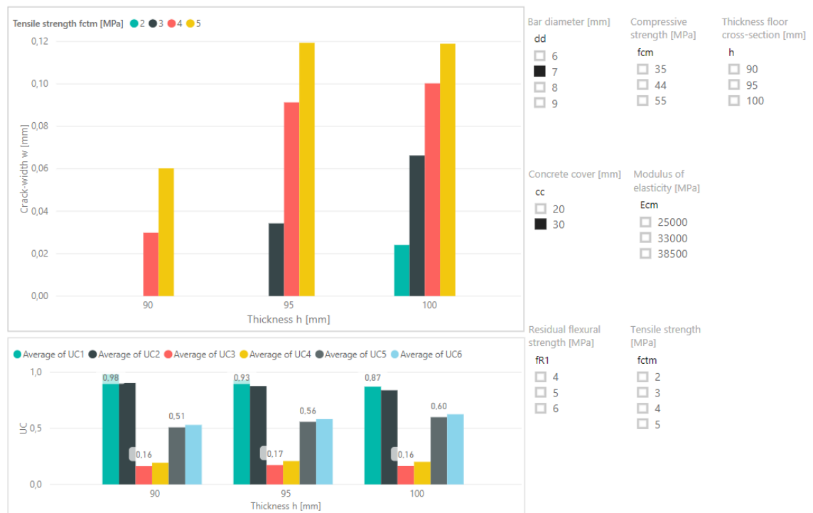
Figure 5.9 Suitable floor thicknesses with a top reinforcement mesh of \phi 7 -100 mm with a concrete cover c = 30 mm, shown in accordance with suitable tensile strengths. Shown possible variants suitable for all UC's \leq 1.0 and w_{max} < 0.12 mm. Top left: max crack-width of the suitable options for different floor thicknesses with a certain tensile strength. Bottom left: average of the ULS unity checks 1-6 for different floor thicknesses. Right: selected parameters bar diameter dd 7 mm and concrete cover c 30 mm; only the possible solutions in accordance with these settings are visible in the diagrams.
