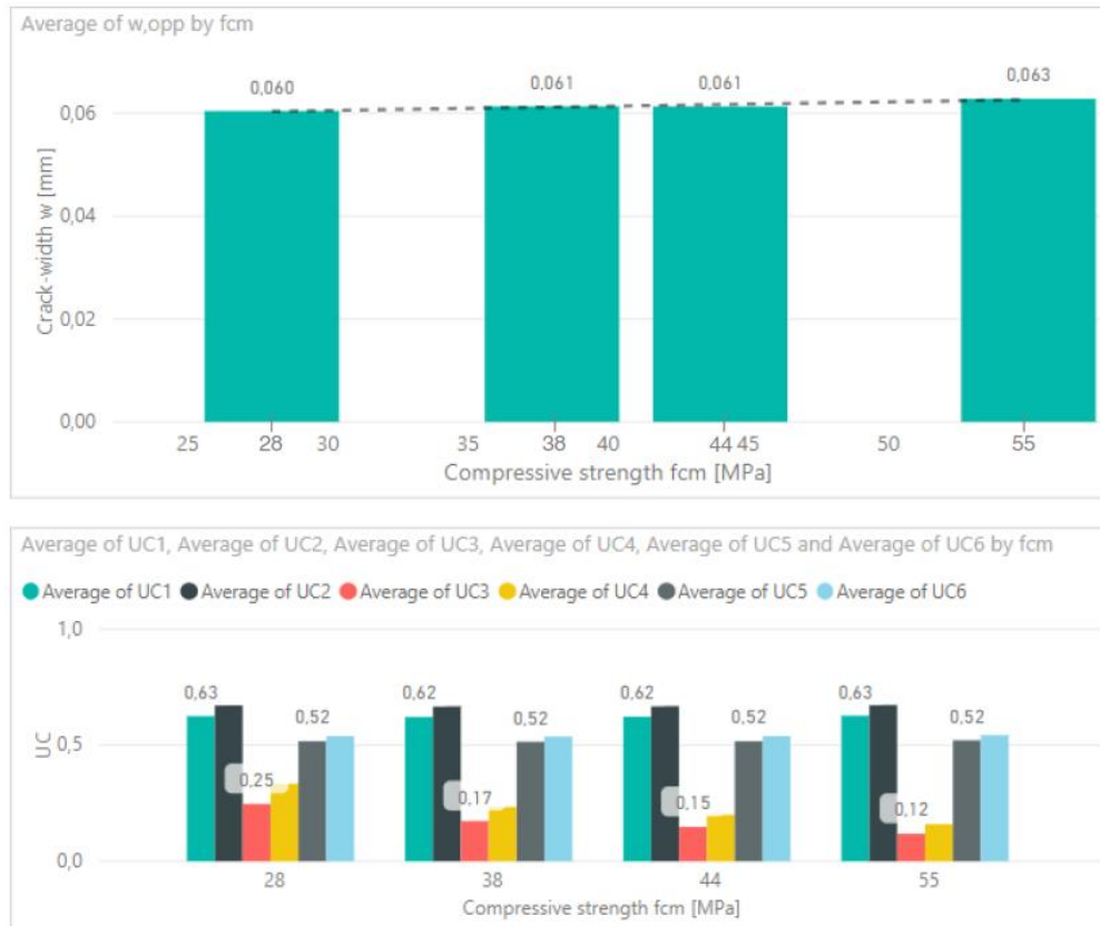
Figure 5.10 Top: average crack-widths for different compressive strengths f_{cm} . Bottom: Average values for the ULS unity checks for different compressive strengths f_{cm} . Compressive strength f_{cm} values of 28, 38, 44 and 55 MPa.
