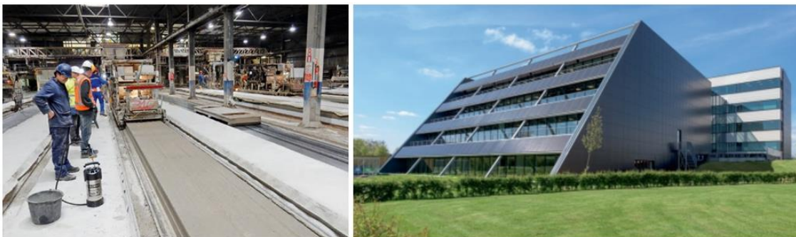
Figure 4.8 Production of the alkali-activated concrete hollow-core slab (left) and the office building in Hengelo in which these slabs have been applied (de Vries, 2017).
