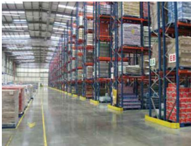
Figure 2.1 Warehouse with back-to-back racking's on a concrete floor (The Concrete Society, 2016).
