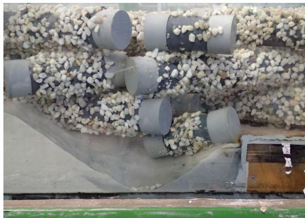
Figure 5.14: Unstable filter layer at time step 5 of experiment R08. The experiment was stopped in order to prevent damage of the ADV2 inside the filter layer.
