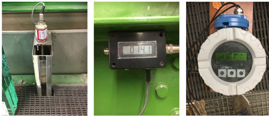
Figure 3.9: The digital water level measurement (left and middle) of the return flow and the discharge meter (right).
