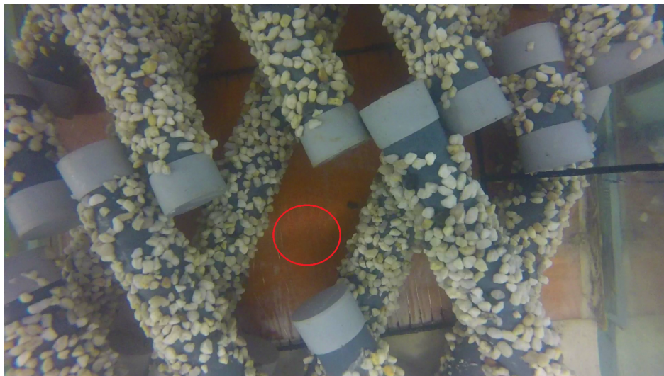
Figure 6.2: Created additional space for the ADV2 device in experiment R05: the distance between two logs is slightly higher than the normal geometry. The place of the ADV2 is depicted by the red circle.
