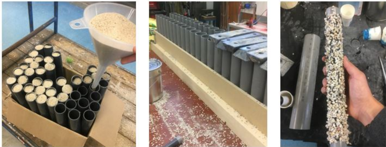
Figure 3.3: Filter material: filling the PVC with sand (left), glueing roughness elements (middle) and final log (right)
