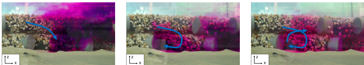
Figure 5.7: Vortex behind (downstream) a log caused by higher flow velocity above the log than behind the log
