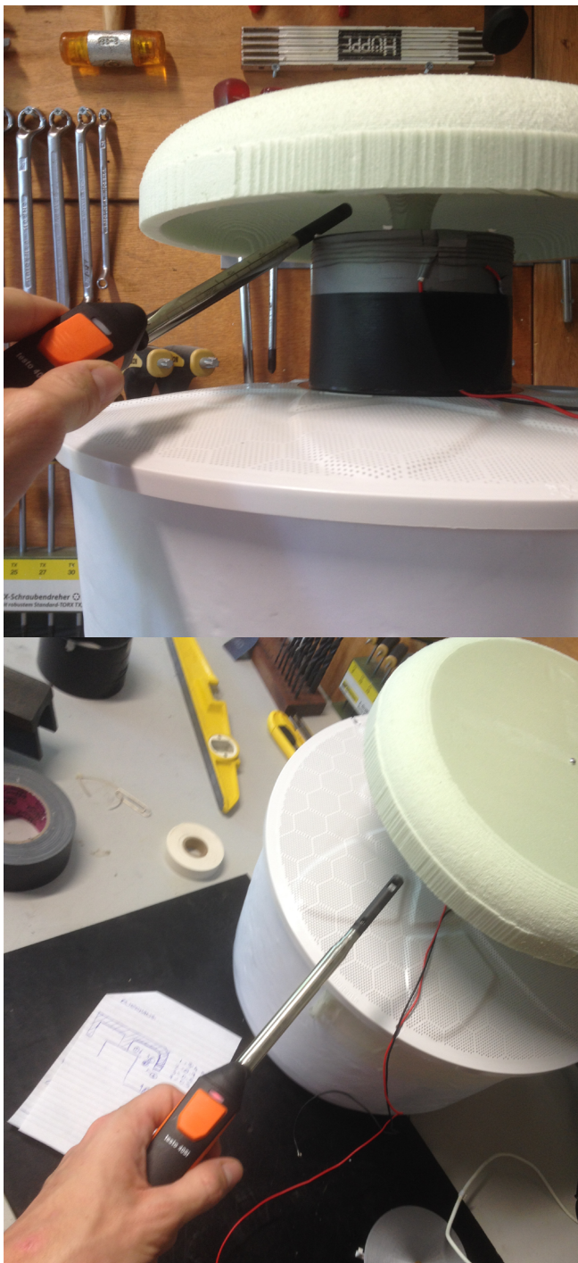
Figure 41: Measuring airspeeds at points around the trap concepts for analysis.
