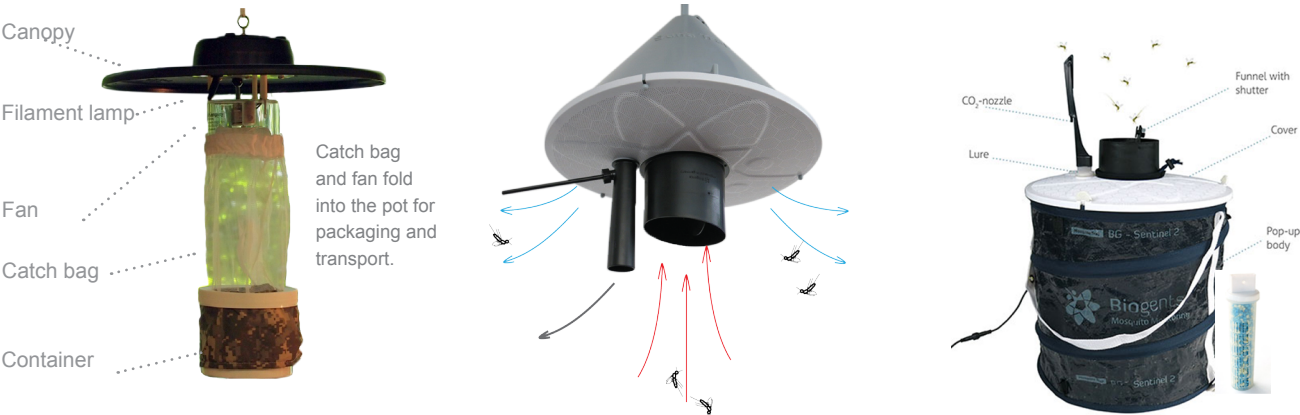
Figure 17: Traps commonly used by researchers. Left: CDC LT. Middle - BG Suna-Trap. Right: BG Sentinel
