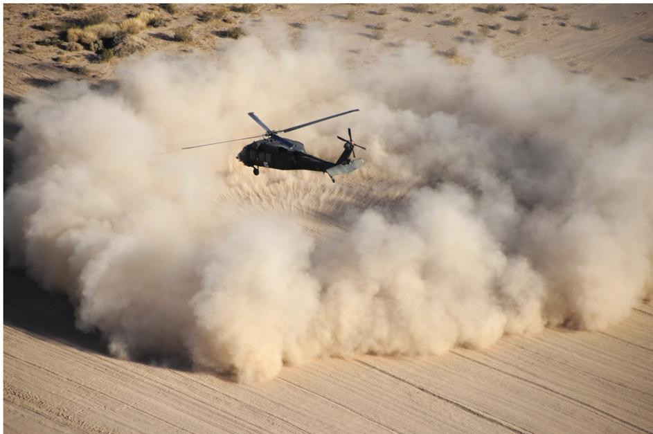
**Figure 2-1:** Aerial view of a brownout forming around a landing helicopter (photo credit: U.S. Army<sup>†</sup>)
