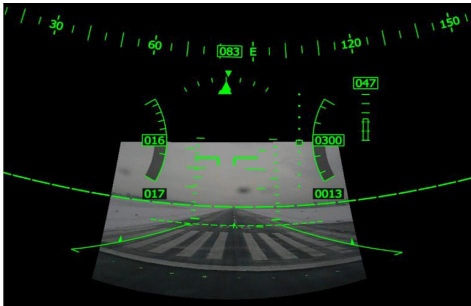
Figure 3-10: Lateral drift indication on landing display by DLR [39]
