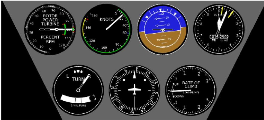
Figure 7-3: Basic instrument panel
