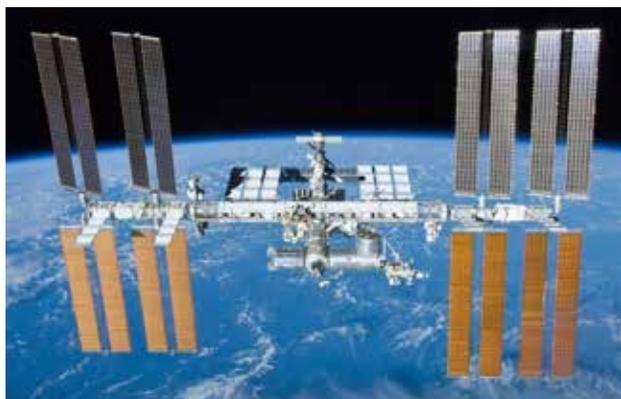
Figure 1. International Space Station with its array of large solar panels. Image courtesy: NASA
