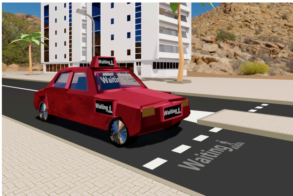
Figure 2. Car combining all five external human–machine interfaces (eHMIs). In the experiment, the car showed only one eHMI at a time. Here, the car has stopped for the pedestrian. The distance between the centre of the car and the camera (pedestrian) is 7 m longitudinal (i.e., parallel to the direction of the road) and 4.5 m lateral (i.e., perpendicular to the road). The white markings on the road were intended to create a pedestrian crossing on the road, without designated priority to the pedestrian.
