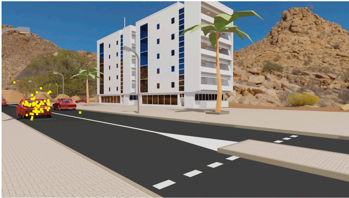
Figure 7. Screenshot of the animation in a straight approach case with the Projection eHMI. The yellow markers represent the gaze positions of all of the participants. The projection in front of the car is difficult to discern from a distance.
