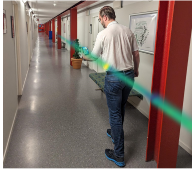
Figure 6.1: Collecting measurements of magnetic field along hallway in university building with a smartphone. The learned magnetic field measurements using the pattern-discovery kernel are displayed. The color corresponds to the learned magnetic field strength, and the opacity corresponds to the confidence of the estimate. As the metallic columns create a repetitive magnetic field pattern, our online pattern-detection algorithm is able to predict the magnetic field variations not only in the walked trajectory but also further down the hall.
