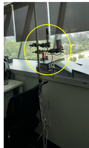
(b): Portables poles with loggers
