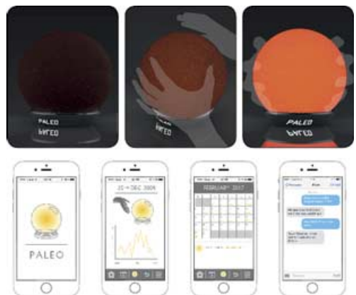
Figure 8. Paleo, inspired by CONVERSATIONS. Retains heat and radiates a warm glow. Sensors emit a brighter light as hands draw close encouraging interaction which in turn wears down the surface over time creating a unique and personalised light silhouette in your home.
