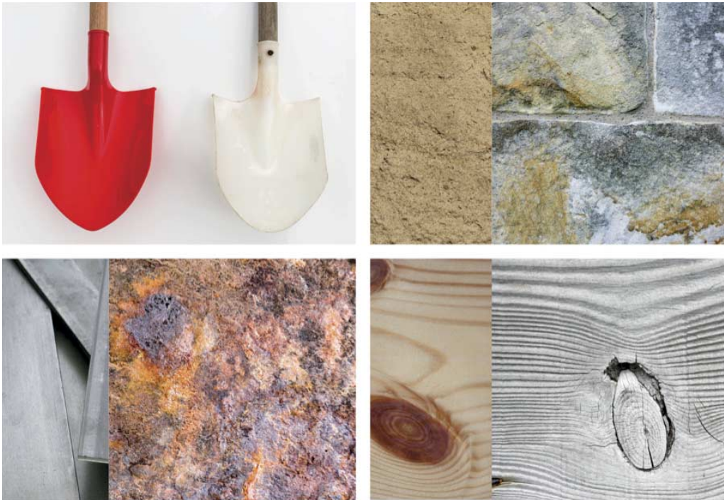
Figure 1. Materials change (clockwise from top left): a plastic spade is severely faded by sunlight (despite it being designed for outdoor use); sandstone develops a rich patina of lichen; wood has lost colour but the surface texture is accentuated after exposure to sunlight and salt from the sea; mild steel reacts with oxygen and water to produce beautiful but fragile rust. In each case the new material is on the left. Except for the spade, the new and old materials are similar but not identical samples.
