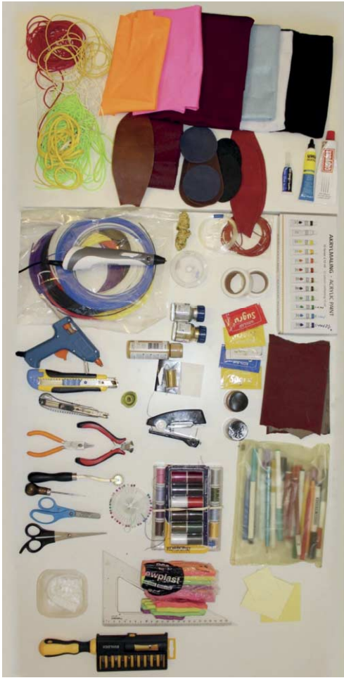
Figure 2. Workshop tool-bag including materials and tools such as fabric, 3D printing pen, patches, Sugru and sewing tools.
