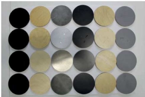
Figure 1. Material sample discs used in study [From left to right; Plastic Gloss, Wood Gloss, Metal, Plastic Matte, Wood Matte and CLEVER material. From top to bottom; Abrasion, Ablation, Impact and Accumulated Dirt.] (Authors own image)
