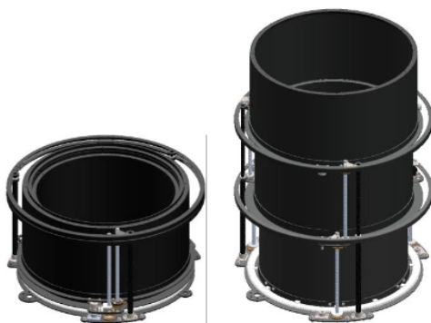
Figure 2.7: Concept of the SSTL telescopic deployment barrel. (Gooding et al., 2018)
