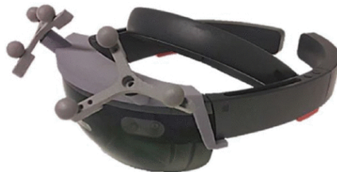
Figure 2.5: Optical tracking spheres can be attached to the HoloLens. The relative location of tracked tools or patients is then known and can be used to display models in the HoloLens. (Meulstee et al.)
