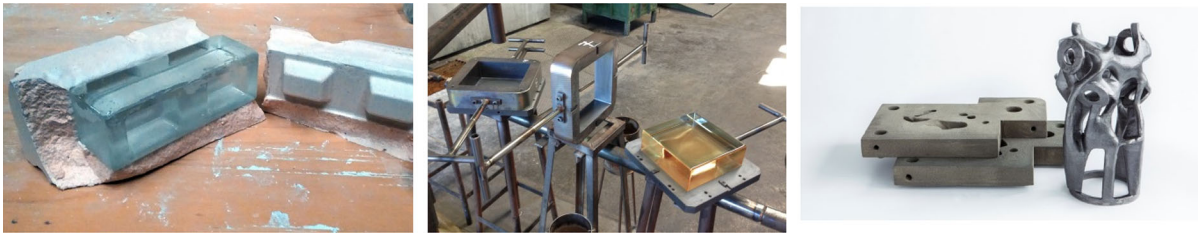
Fig. 19 From left to right: Disposable low-precision mould, open high-precision metal moulds (Oikonomopoulou et al. 2020), 3D-printed sand moulds (image credits: ARUP/Davidfotografie)
