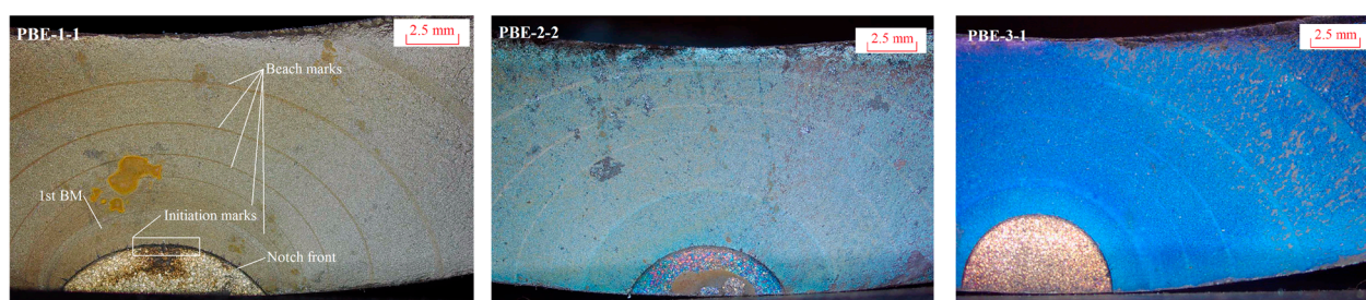
Figure 6. Photographs of surface crack growth in metallic pipes marked by the beach mark (BM) technique [12].
