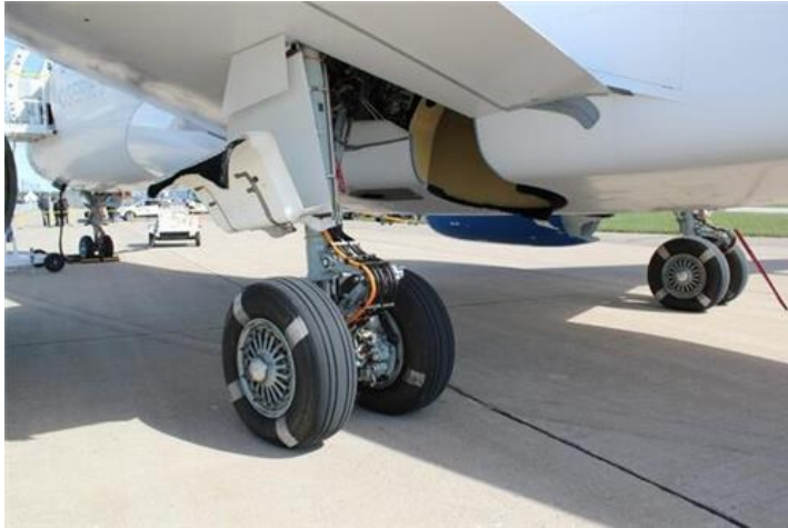
Figure 7.9: Image showing the landing gear configuration on the Bombardier C Series. flickr.com
