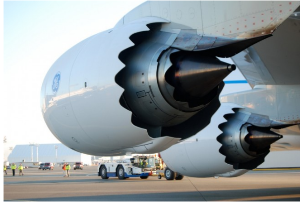
Figure 13.5: Serrated edges, chevrons, on the rear of GENx turbofan engines. wired.com
