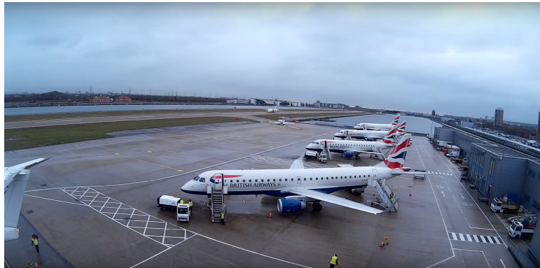
Figure 17.5: Image showing the aircraft line-up at LCY gates. All aircraft are facing the taxiway, instead of the terminal [145].
