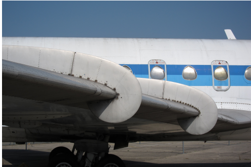
(a) Wing fences on a Sud Aviation SE 210 Caravelle. commons.wikimedia.org
