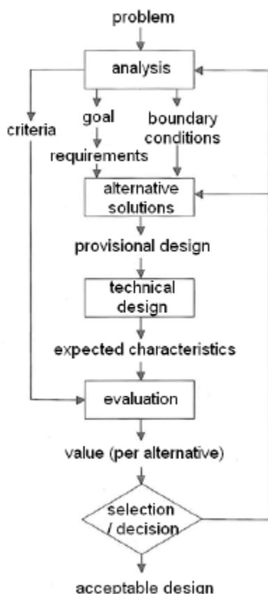
Figure 11: Visualization of the Delft Design method (Voorendt, 2015)
