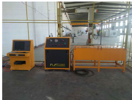
Fig. 12. Short-term burst pressure test system.
