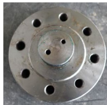
Fig. 13. Configuration of the end cap.
