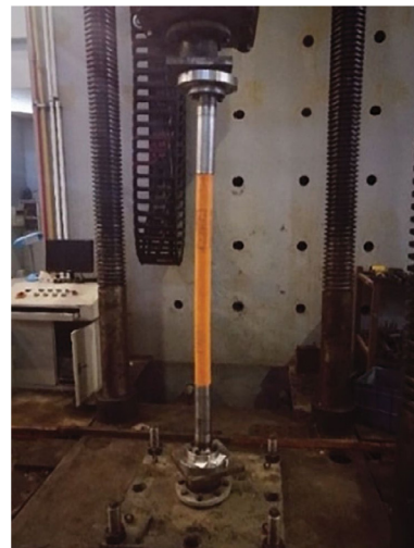
Fig. 8. Tensile test of a specimen.
