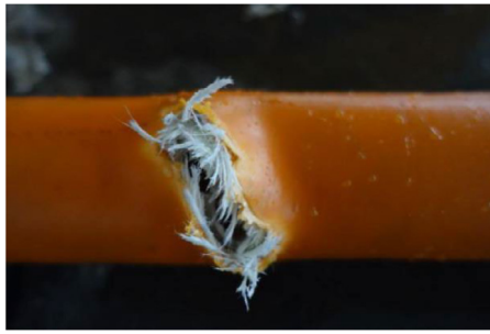
Fig. 15. Detail of a burst position.
