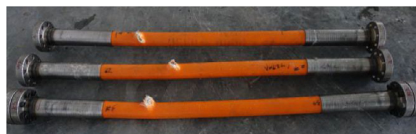
Fig. 14. Test specimens after burst.
