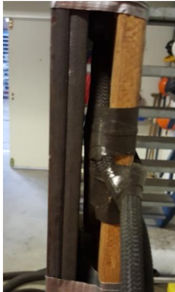
Figure 28 - Test plate set-up with induction coil attached
