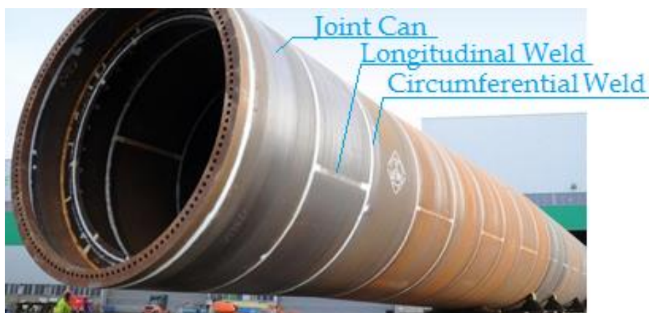
Figure 49 - Tower assembly and weld types
