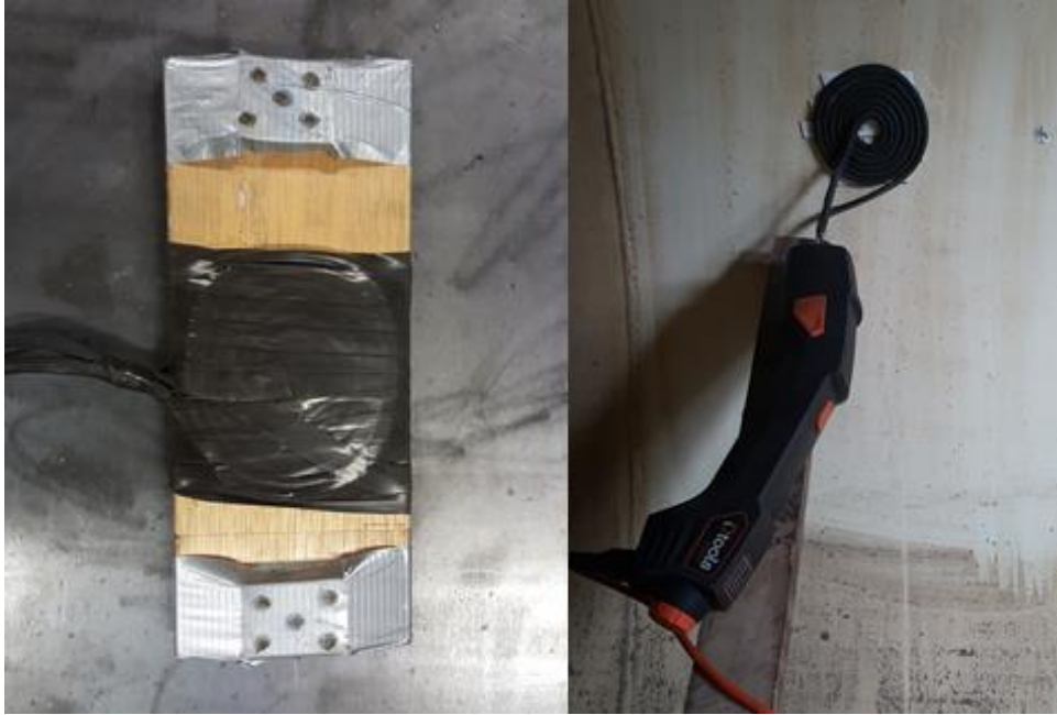
Figure 18 - (a) Heating coil in frame, (b) Induction unit with unwrapped coil
