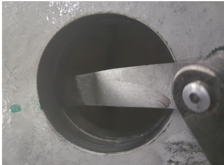
Figure 44 - Feeler gauge testing in sample slip-joint
