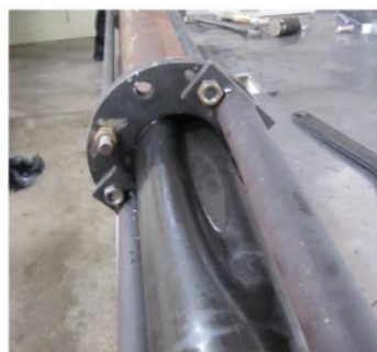
Figure 52 - Shrink buckling in pipe liner
