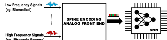
Fig. 1: Illustration of sensory signal processing pipeline using a general purpose analog front end and SNN.
