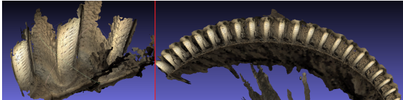
Figure 21. The left image shows a small Poisson reconstruction which has more detail than the larger reconstruction on the right. The base settings for Poisson reconstruction lead to larger interpolation and less detail, which can be changed for high quality large reconstructions.
