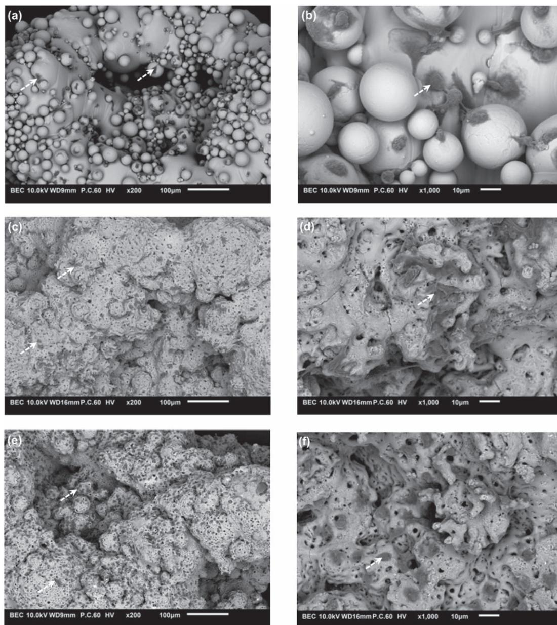
**Figure 3.** SEM images of the human monocyte-derived macrophages (indicated by the white arrows) attached on: (a), (b) SLM implants; (c), (d) SLM PEO implants; (e), (f) SLM PEO+Ag implants after 4 d of culture.
