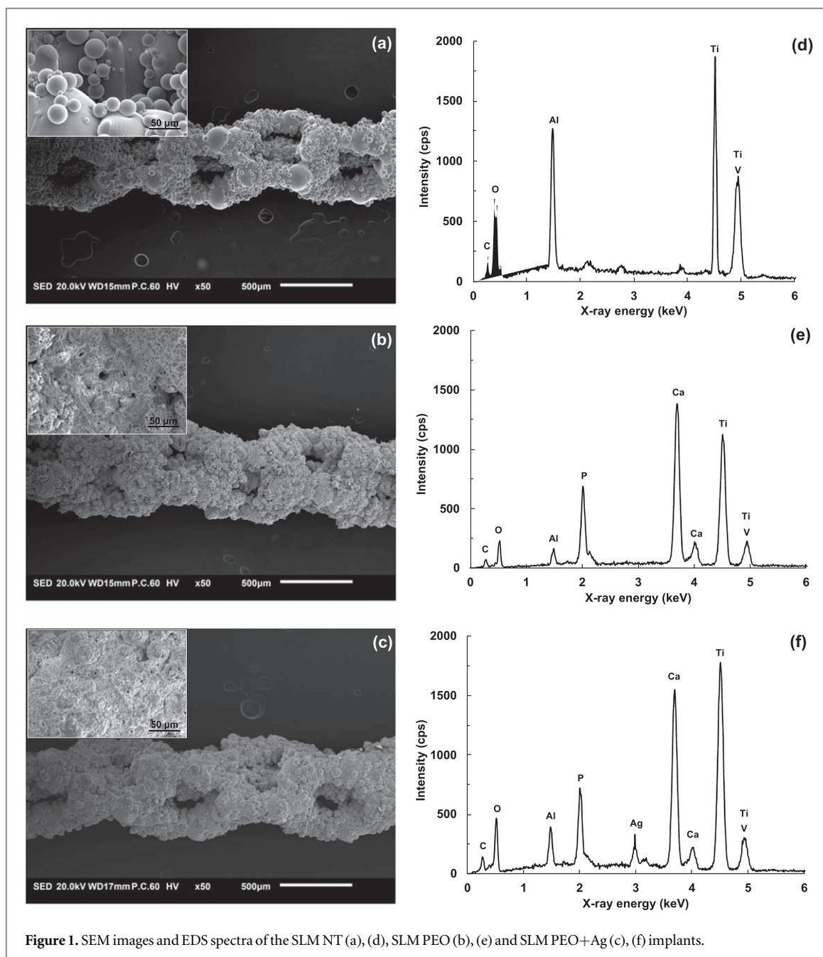
**Figure 1.** SEM images and EDS spectra of the SLM NT (a), (d), SLM PEO (b), (e) and SLM PEO+Ag (c), (f) implants.
