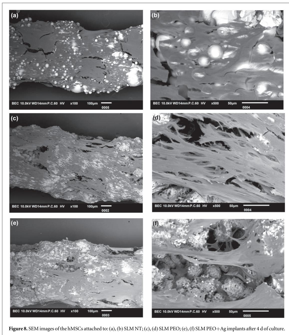
**Figure 8.** SEM images of the hMSCs attached to: (a), (b) SLM NT; (c), (d) SLM PEO; (e), (f) SLM PEO+Ag implants after 4 d of culture.
