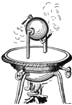
FIGURE 2.17 - ILLUSTRATION OF THE WORKING PRINCIPLE OF THE AEOLIPILE (KNIGHT'S AMERICAN MECHANICAL DICTIONARY, 1876)
