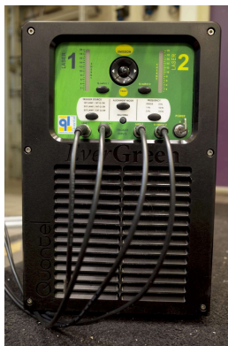
Figure 4.9: Power supply, cooler and control unit for the Quantel Evergreen laser
