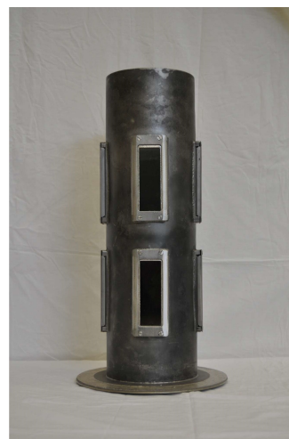
Figure 3.9: The flametube, showing its quartz windows on three sides
