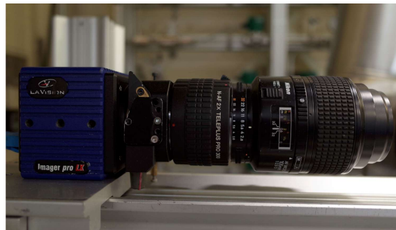
Figure 4.12: The Lavigation Imager Pro LX 16 camera with an f_{\text{effective}}=210 \text{ mm} lens, used for the zoom-case
