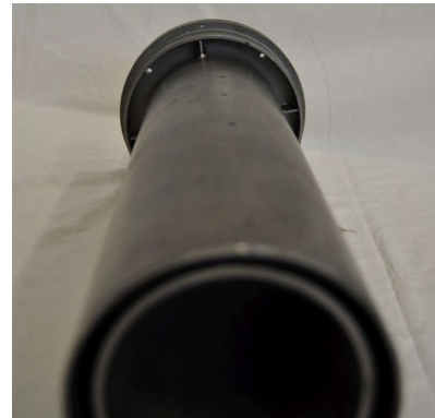
Figure 3.12: The moveable exhaust pipe, showing the separation between the cooling and combustion flow
