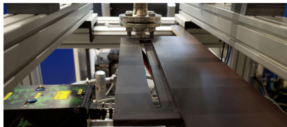
Figure 4.20: A black wooden plank with a slit, used to prevent interference from reflections from the bottom of the cylinder
