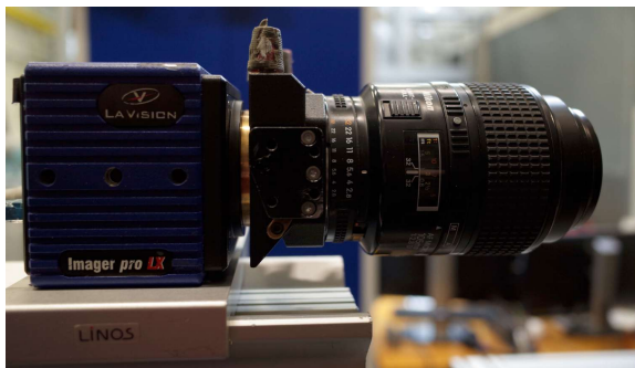
Figure 4.11: The LaVision Imager Pro LX 16M camera with an f=105 \text{ mm} lens
