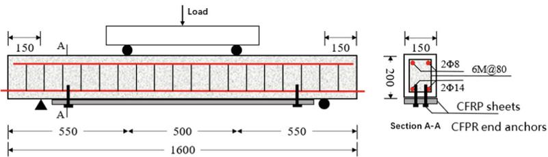
Fig. 1. Dimensions and reinforcement details of RC beams.
