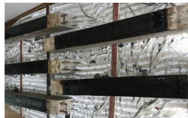
(c) Finished RC beams reinforcement.
