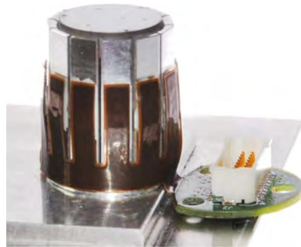
(a) The ASML/PI TSA mounted in its housing. This housing acts not only as a means to mount the sensor and the actuator, but it also reduces the displacement sensitivity to environmental temperature changes, by placing the electrode in the thermal centre. (The housing and the fingers expand equally, reducing the electrode motion due to environmental temperature changes.)
