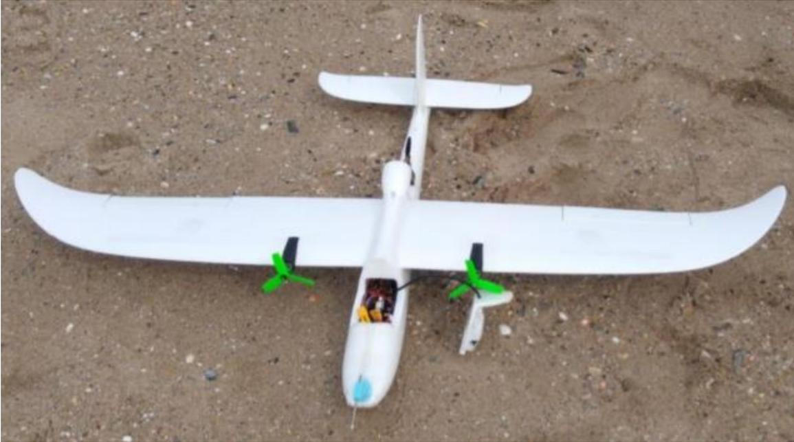
Figure 3.3 Aircraft used in flight test campaign [13]
