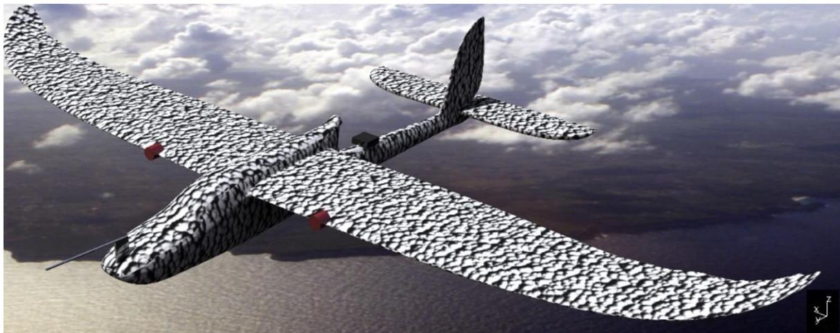
Figure 5.13 Rendering of the test aircraft including all components in Catia V5
