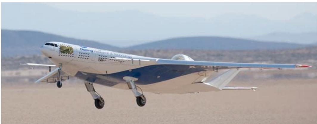
Figure 2.4 X-48C remotely piloted liftoff at Edwards air force station for its first test flight [10]
