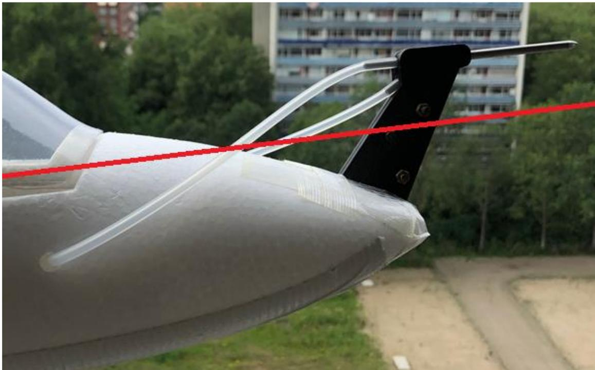
Figure 3.8 Pitot tube mounting location and tube routing. The approximate free stream velocity direction during 18 m/s cruise is shown in red
