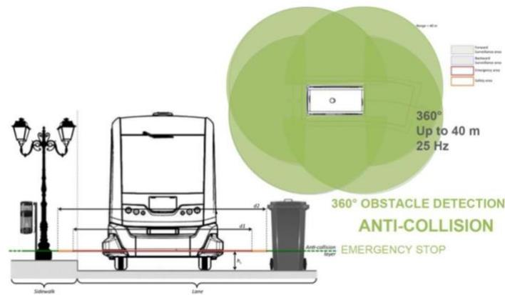
Figure 3.11. The static dimensions of the Easymile (Boersma, Van Arem, Rieck, 2018)
