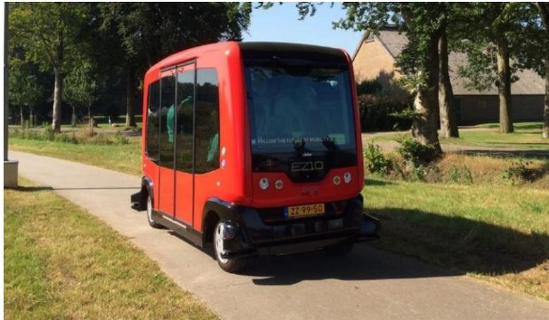
Figure 6.3: The Easymile EZ10 shuttle used in the Appelscha project (Boersma, van Arem, and Rieck, 2018)
