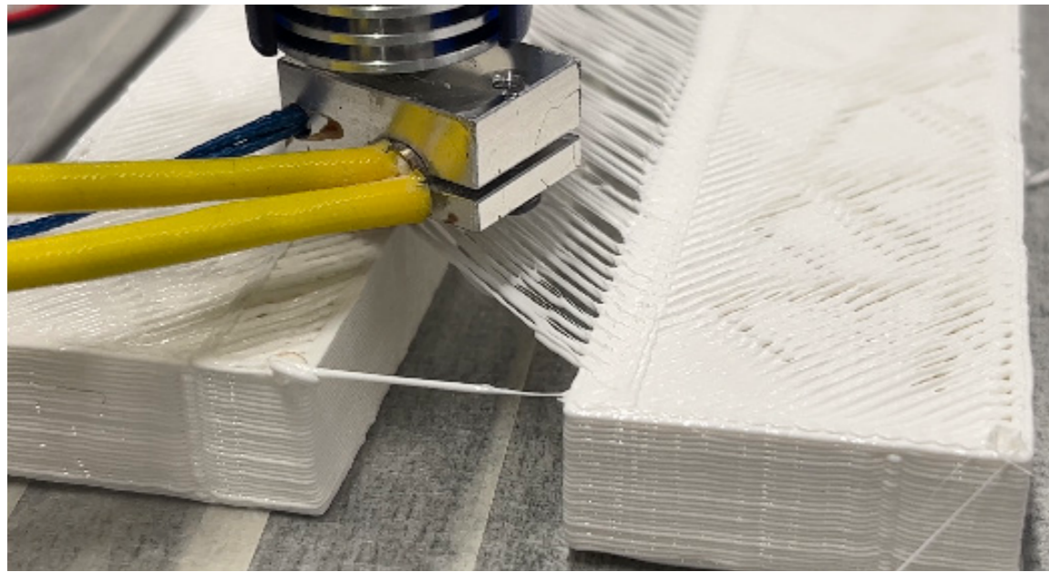
Figure 70: The most difficult layer to print with the overhang, the first infill layer. The connection with the surface of the 2 voxels is key for the material to stay up.
