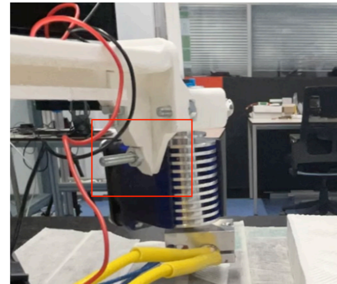
Figure 68: The cooling fan is forcefully turned to the side of the shoulder so it does not clash with the previous voxel.
