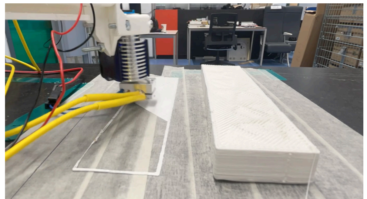
Figure 69: Screenshot of the timelapse of the second voxel printing during the stacking test. The second voxel was placed approximately 20 mm away from the first one.
