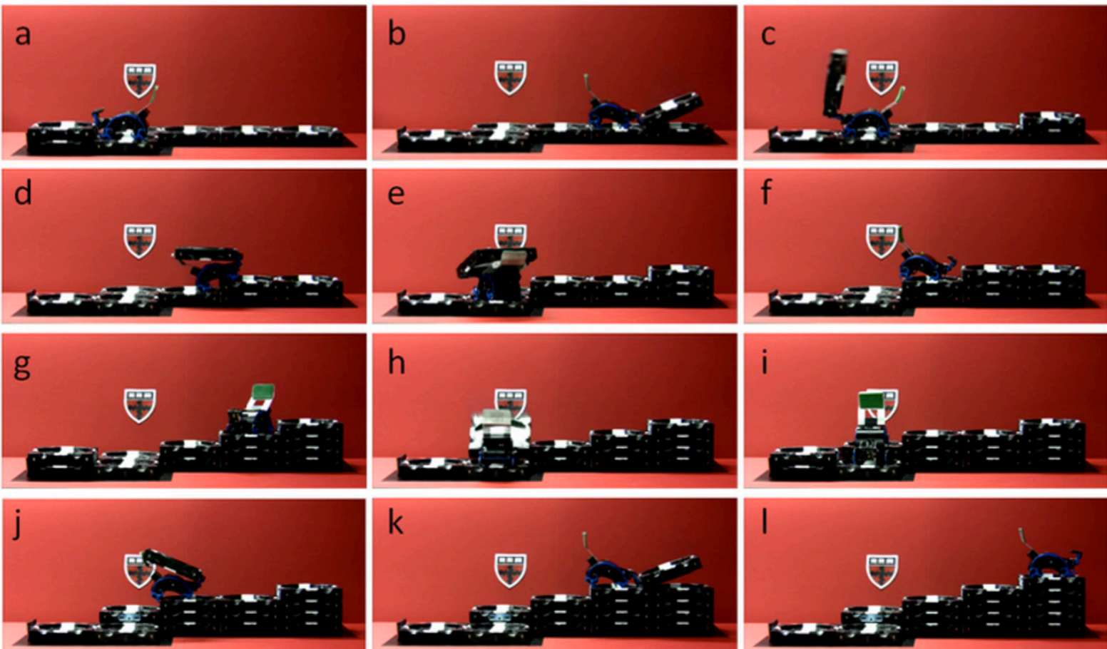
Figure 23: Forward and backward printing strategies used by the robot to reach location A. The sequencing of the blocks are numbered.
