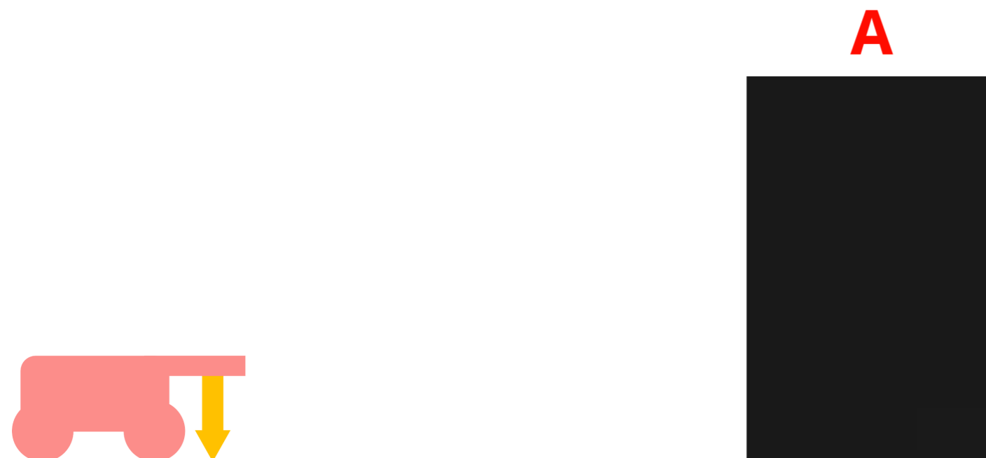
Figure 20: The robotic builder (on the left) that has the goal to reach a specific point A on top of a structure. It must reach the structure by building its own ramps.
