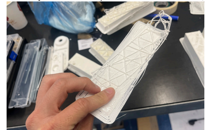
Figure 63: Failed print during test print 6, same aggressive misalignment as in print test 3.
