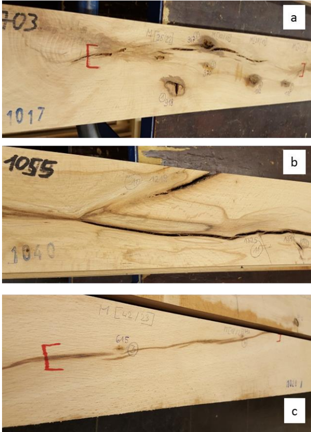
Figure 2: Typical wood defects: a) knots, pith and fibre deviation, b) cracks, c) slope of grain, pith and discoloration
