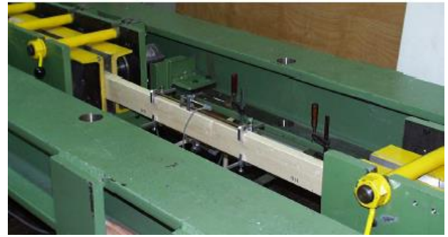
Figure 3: Testing device according to DIN EN 408 [11].
