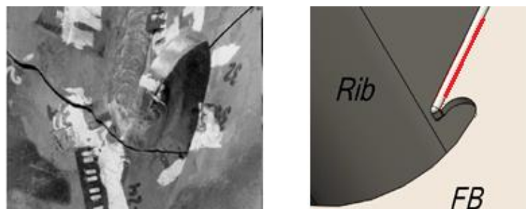
Figure 1.2 Fatigue cracks from weld toe to trough and crossbeam (Kolstein H. , 2007)
