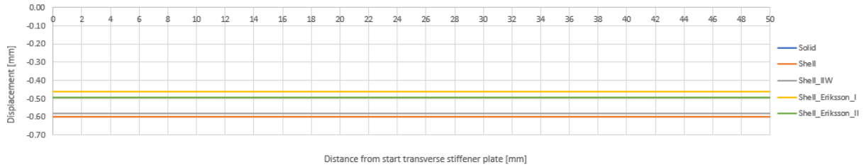
Figure J 0.23 Deformation U1 (X-direction), loading type IV: combination in-plane and out-of-plane I, new variant
