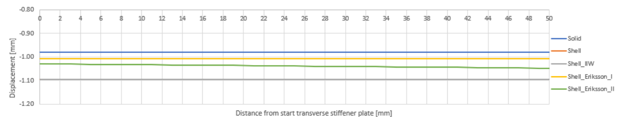
Figure J 0.21 Deformation U3 (Z-direction), loading type III: out-of-plane II, new variant
