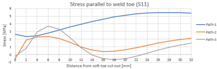
Figure E 0.5 LP2: Stress parallel to weld toe for path 1,2 and 3 solid FE model
