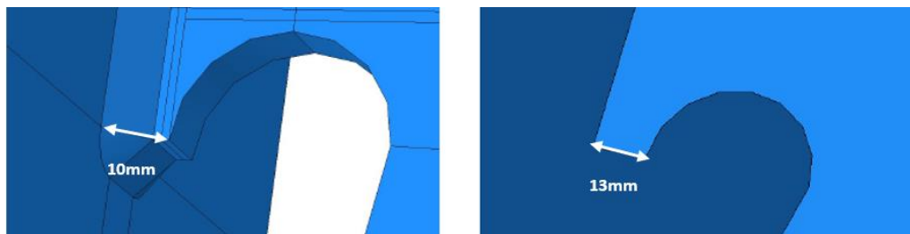
Figure 6.67 Local geometry soft toe, solid (left) and shell (right)
