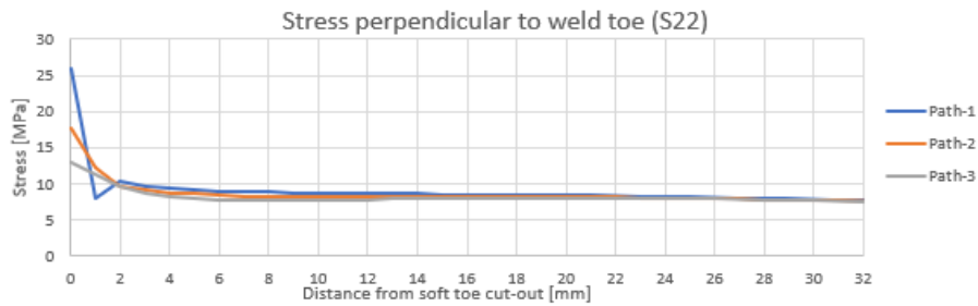
Figure E 0.9 LP2: Stress perpendicular to weld toe for path 1,2 and 3 shell FE model
