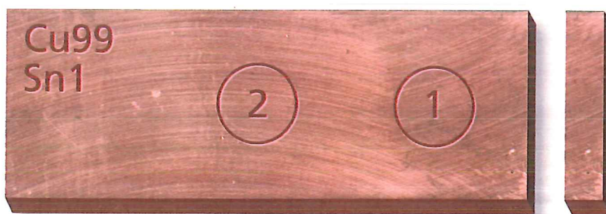
Fig. 1: Schematic overview of a copper 99% and tin 1% sample with both circular spots where XRF measurements will take place. At the end of the sample a cross section was made for possible reference. Spot 1 and 2 will be referred to in the tables as ‘before brazingspot 1’, ‘before brazingspot 2’.
