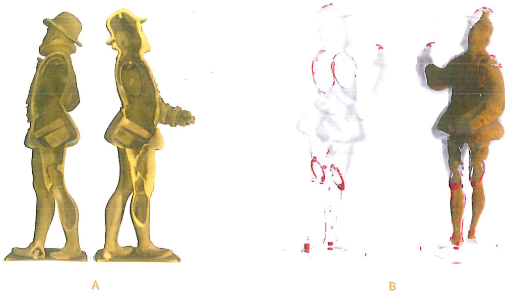
Fig. 2: Neutron tomography data of the Striding Nobleman . (a) Alloy/metal distribution. (b) Distribution of soldered joints (left) and hollow parts (right).
