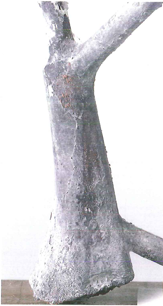
Fig. 23: The casting result of investment material that was not ground to flour.
