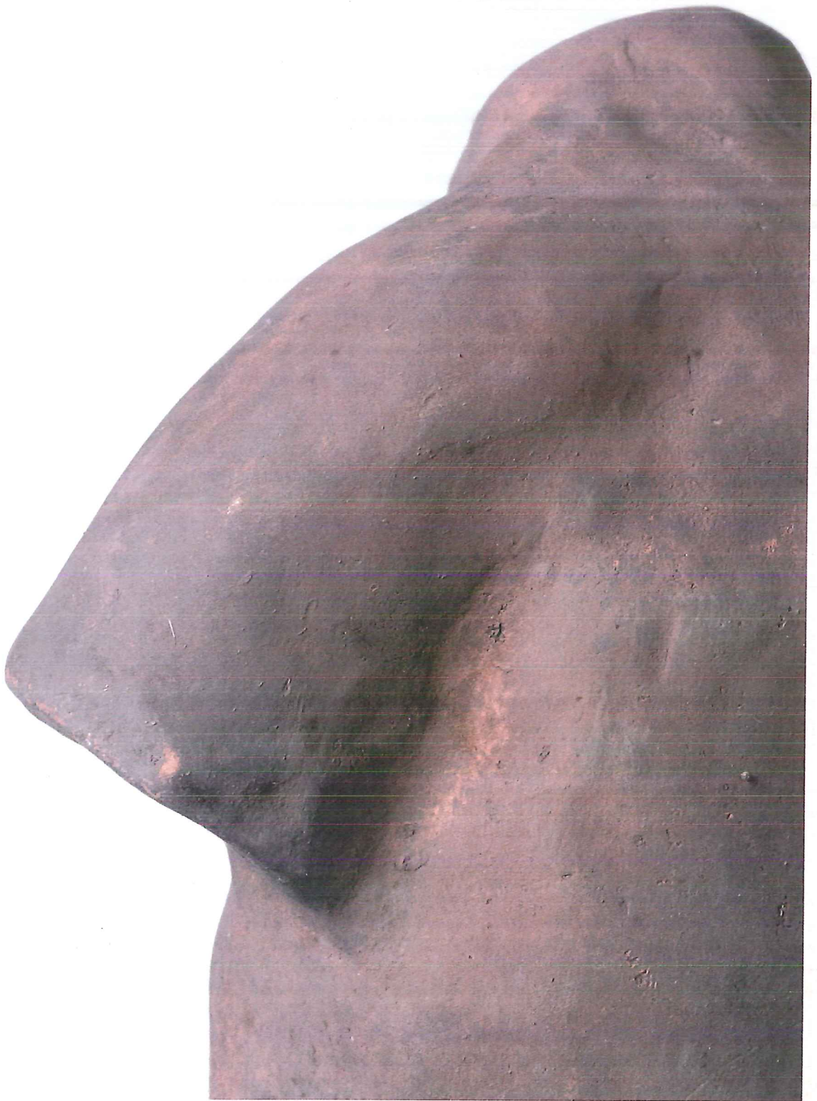
Fig. 22: Detail of 3.7 model showing the superbly soft finish of the bronze after removal of the casting skin.
