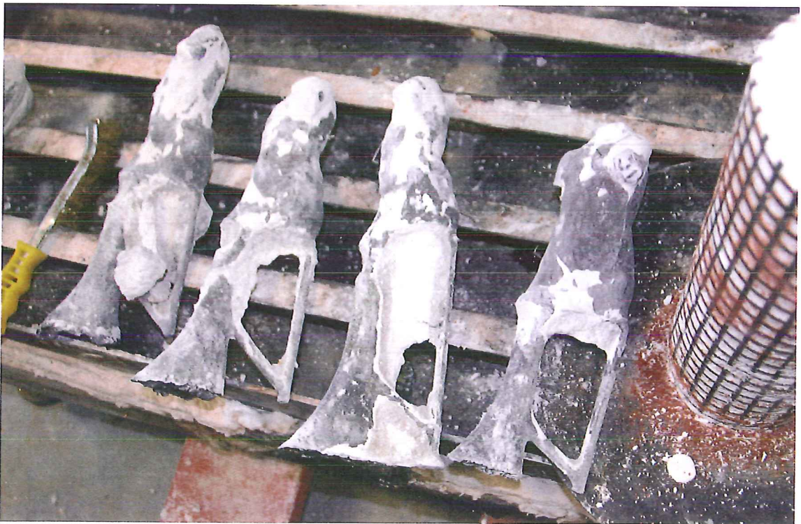
Fig. 17: The casting results still partially covered with the investment material. Note the colour change in the investment material closer to the cast metal.
