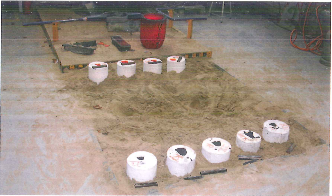
Fig. 12: The various investment moulds are placed in sand.
