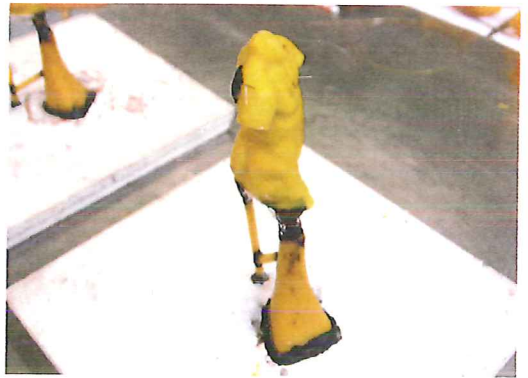
Fig. 5: The wax model placed on one conical sprue (feeder) and one vent.
