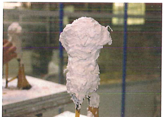
Fig. 7: The second coarser material of the same ingredients of the investment. Note that the sprue and vent are not covered with the fine detailed first layer of the investment.
