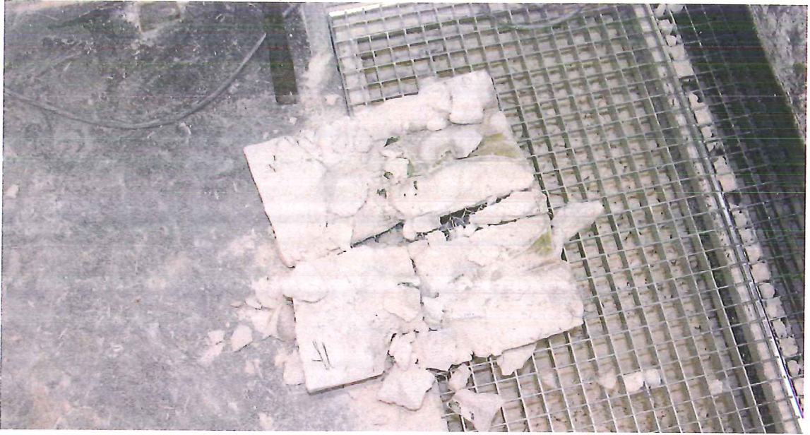
Fig. 16: After sufficient cooling, the investment is removed from the cast bronze.
