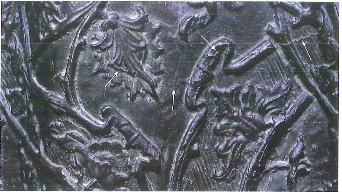
Fig. 9b: Sigmund der Münzreiche , detail of the back of the torso showing an arbitrary fin in the centre of the photograph going to the right caused by the shrinkage of the mould. Small balls can be seen throughout the bronze, for example, under the leaf close to the start of the crack. Cenotaph Maximilian I, Innsbruck. (photograph by G. Steinmetzer).
