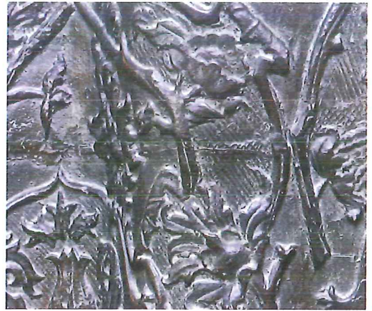
Fig. 9a: Sigmund der Münzreiche , detail of the back of the torso showing a straight fin caused by modelling and small metallic balls in the middle of the picture, indicating that no finishing with hammers and punches of the metal took place. Cenotaph Maximilian I, Innsbruck (photograph by G. Steinmetzer).
