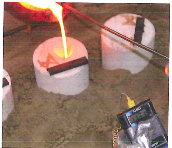
Fig. 15b: A pyrometer shows the casting temperature.
