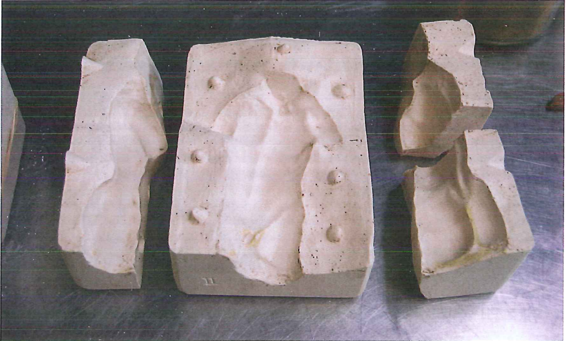
Fig. 1: The plaster mould in three parts..
