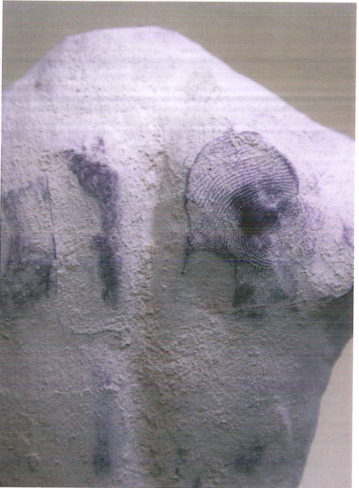
Fig. 18: The final casting result of a fingerprint in metal.
