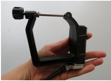
(a) The measurement oarlock of PowerLine [41]. This sensor belongs to the "standard" PowerLine measurement system.
