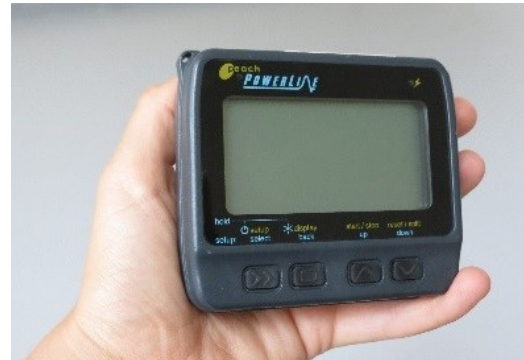
(b) The logger of the PowerLine system records the sensor values at a sample frequency of 50 Hz. It has several real-time functions, used as feedback in the boat. The logger has to be connected to the computer to read out the data, using the PowerLine software.
