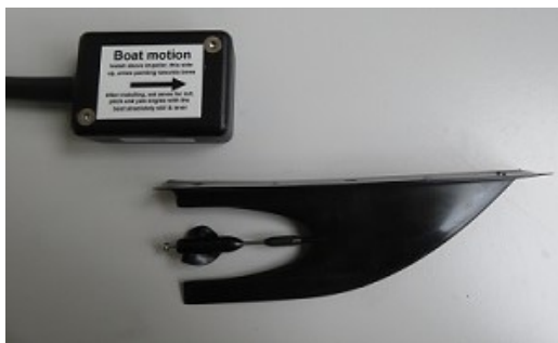
(a) The IMU (top) and the impeller (bottom) of the PowerLine system [41]. The IMU is to be placed horizontally on a flat surface on the hull. The impeller is attached to the bottom of the hull.
