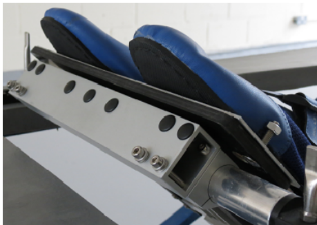
(a) The foot stretcher force sensor of the PowerLine system [41].
