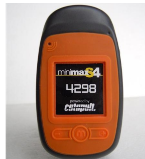
(b) The MiniMax S4 is a sensor that combines GPS with accelero-, gyro- and magnetometer data. It is used to measure the motions of the rowing boat with a frequency of 100 Hz [34]. The device is attached to the inside of the hull and used during the M4X race.
