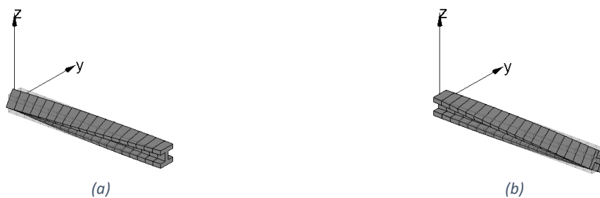
Figure D-4: Rotation around the x-axis for node 1(a) and node 2(b)
