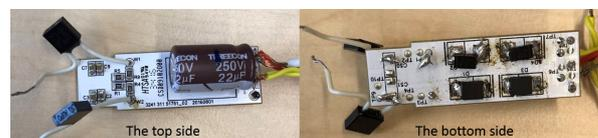
Figure 1.3: A practical driver PCB's on both ends of a TLED tube
