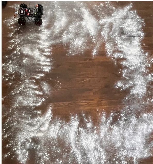
Figure 7.1: Experimental low-friction scenario created with a layer of flour on a wooden floor surface.
