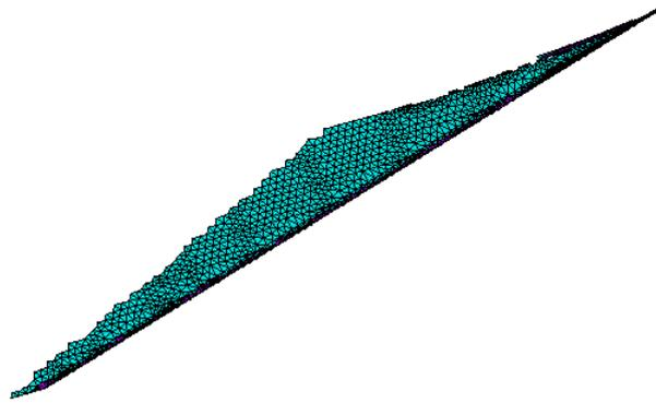
Figure 5.21: Elements that are assigned TPS area CMC
