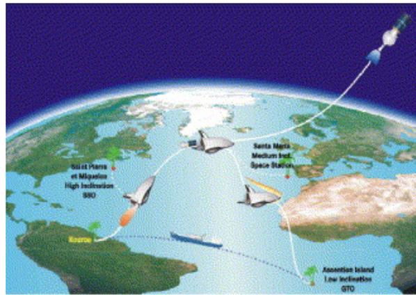
Figure 2.7: Mission profile of the SOH for three different target orbits [5]
