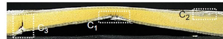
Fig. 3.3 Damage zones on the laminated composite sandwich panel after underwater blast loading (Wei et al., 2013a).
