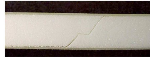
Fatigue fracture of PMI 51 S foam core SSC-463 INSPECTION TECHNIQUES FOR MARINE COMPOSITE CONSTRUCTION AND NDE
