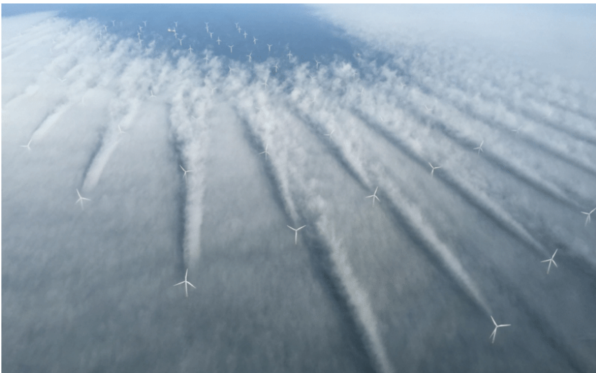
Figure 1.2: A photograph of an offshore wind farm in Denmark in foggy conditions, which clearly shows the wakes behind the turbines. The downstream rows of turbines experience lower wind speeds and higher turbulence intensities as a result of the operation of the upstream turbines. Source: Bel Air Aviation Denmark.
