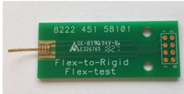
Figure 1.4: The flexible polyimide interconnects device with the contact pad chip mounted on a PCB that was fabricated in a previous project.
