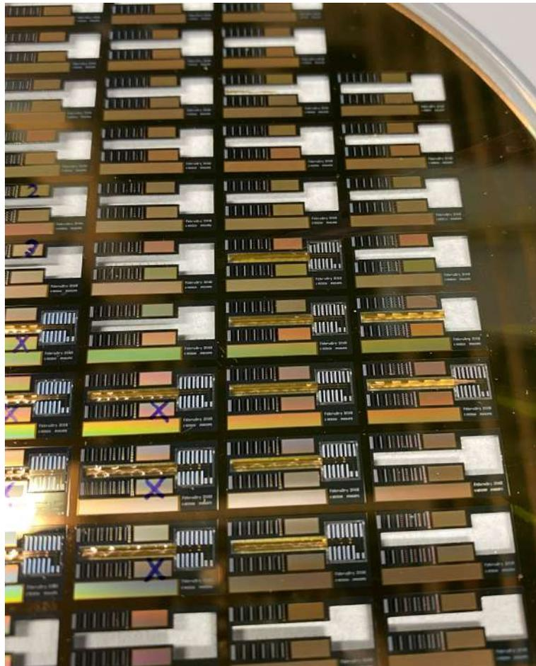
Figure A.1: Previously fabricated F2R interconnects, some samples are already taken out of the wafer for experiments
