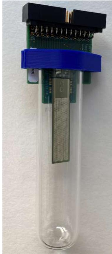
Figure 3.20: A sample mounted on the interconnecting PCB supported on the vial and fixed by the designed cap
