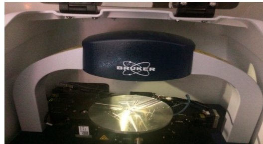
Figure 19. Image of a Stylus Profiler (DektakXT).
